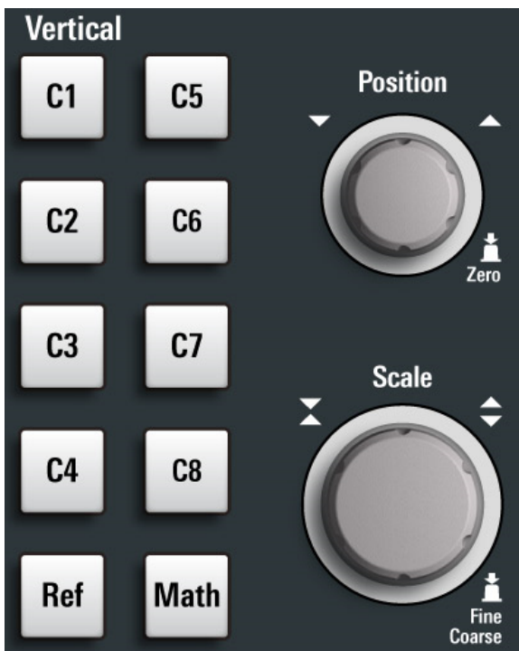
Figure 5-5: Vertical controls of R&S MXO 5 with 8 input channels
