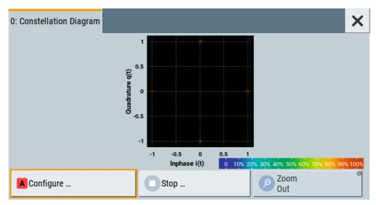
The "Constellation Diagram" displays the 3GPP FDD signal.
