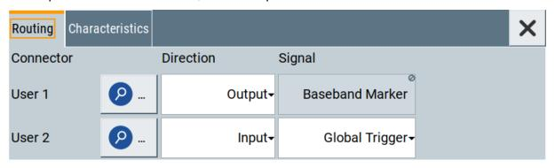
Figure 6-5: Signal mapping to the global connectors
