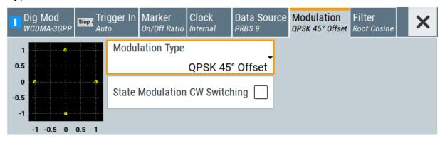
Figure 6-4: Display of the used modulation type
