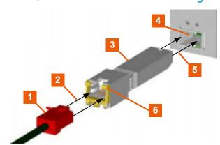
Figure 4-1: Connecting to the IP Data interface
