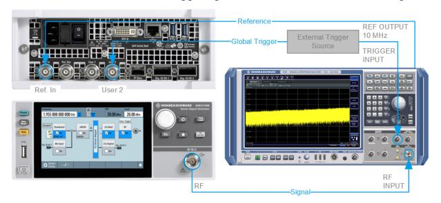
Figure 6-6: Simplified representation of a test setup\*\*
