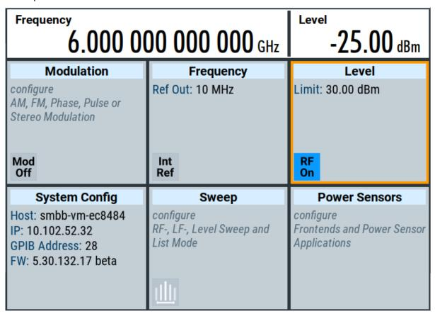
Figure 6-1: Generating an unmodulated signal
