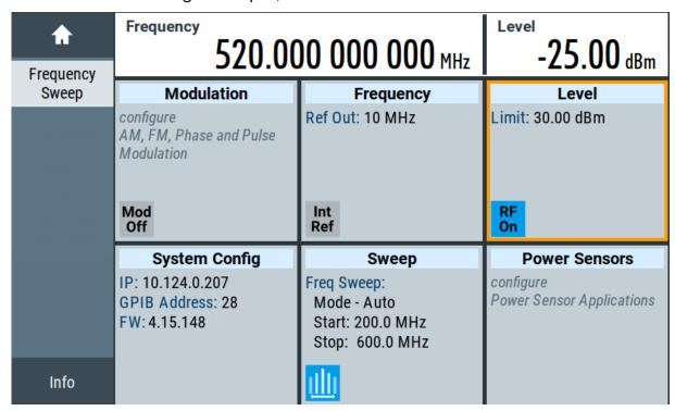
Figure 6-2: Generating a frequency sweep signal
