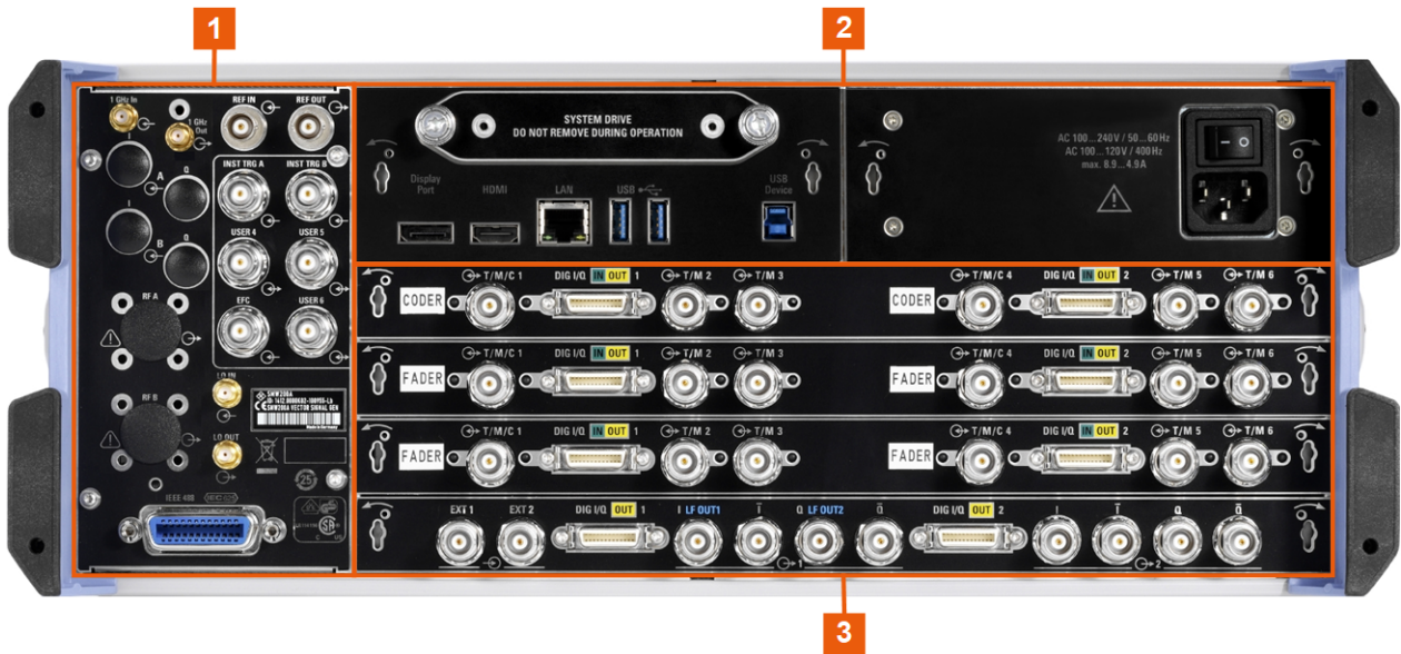
Figure 5-3: R&S SMW200A rear panel connectors (R&S SMW-B10/-B13T)
