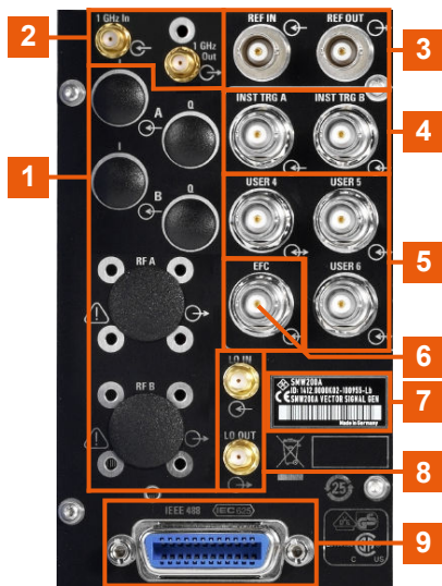
Figure 5-4: Connectors for multi-purpose RF signals and remote control
