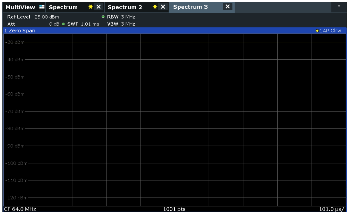
Figure 6-7: Time domain display of the calibration signal
