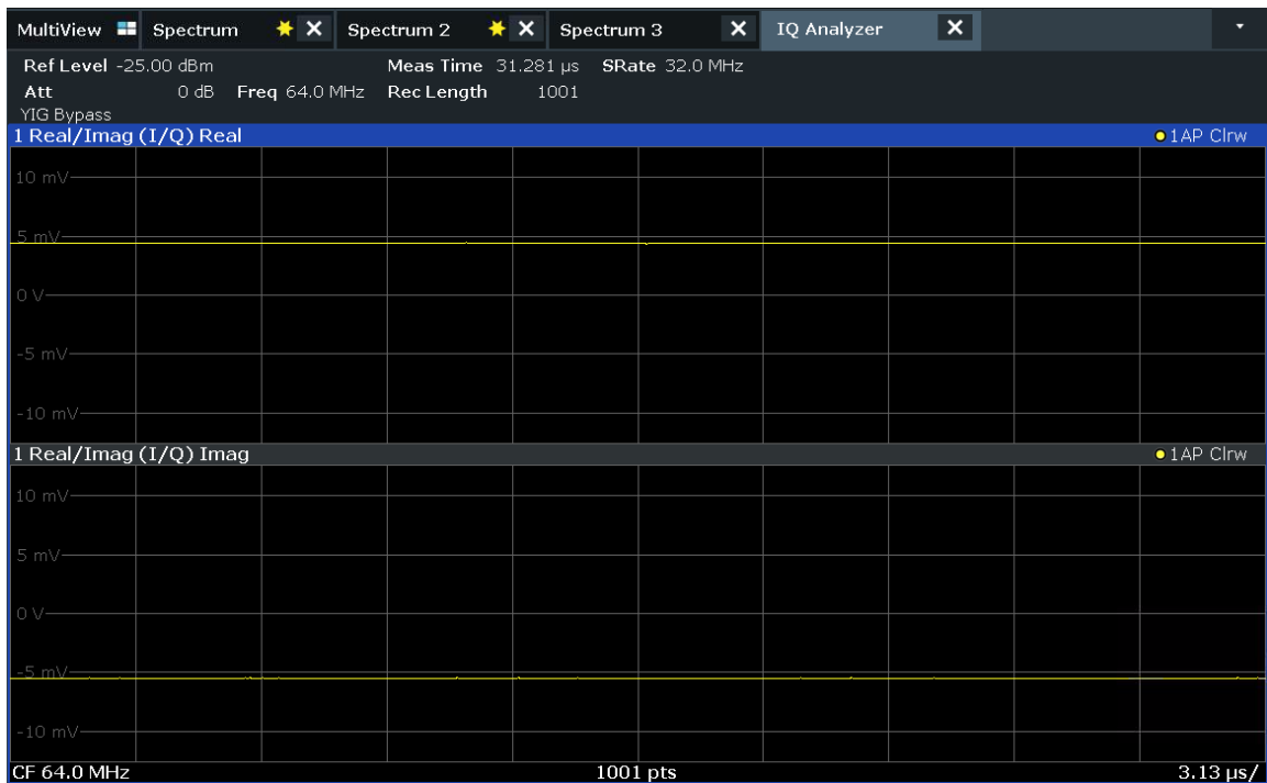
Figure 6-8: Inserting a Real/Imag diagram for I/Q analysis
