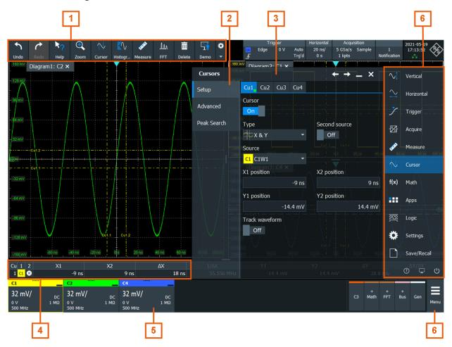
Figure 6-6: Control elements on the touchscreen
