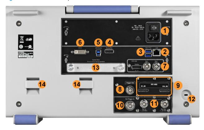
Figure 5-2: Rear panel of R&S RTO
