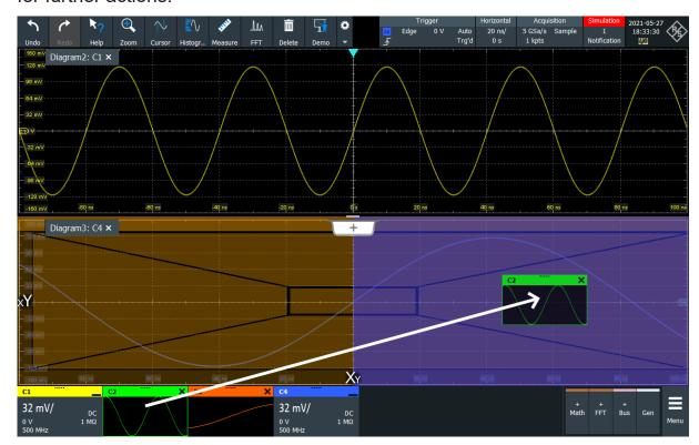
3. To change the size of a diagram, tap the handle between two diagram frames and drag it to the required position.
