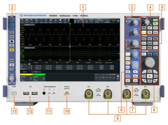
Figure 5-1: Front panel of R&S RTO2044 with 4 input channels
