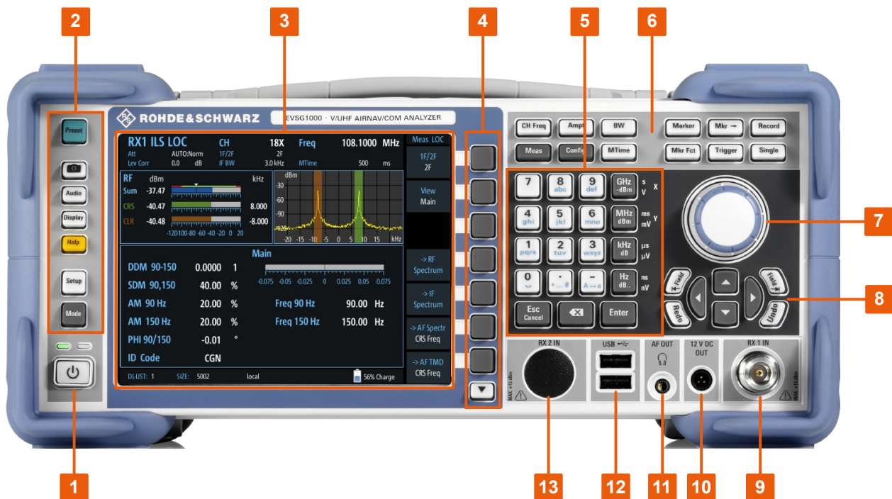
Figure 5-1: R&S EVSG1000 - Front panel view
