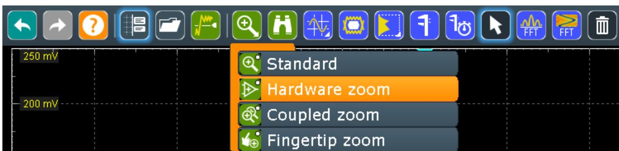
A little triangle in the lower right corner of the icon means, that a menu is available where you can select the required function.
