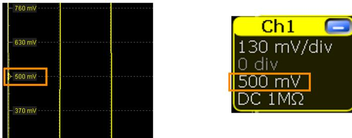
This value is also indicated in the signal icon for channel1 (3rd row). If you press the [Ch1] key, the "Vertical" settings dialog box also displays the "Offset" value. The offset is the DC component of the signal.
