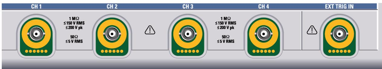
The input connectors are provided with a special Rohde & Schwarz active probe interface, and they are BNC compatible. Thus, the instrument can automatically detect passive probes with standard BNC connector and active Rohde & Schwarz probes having the Rohde & Schwarz probe interface.
