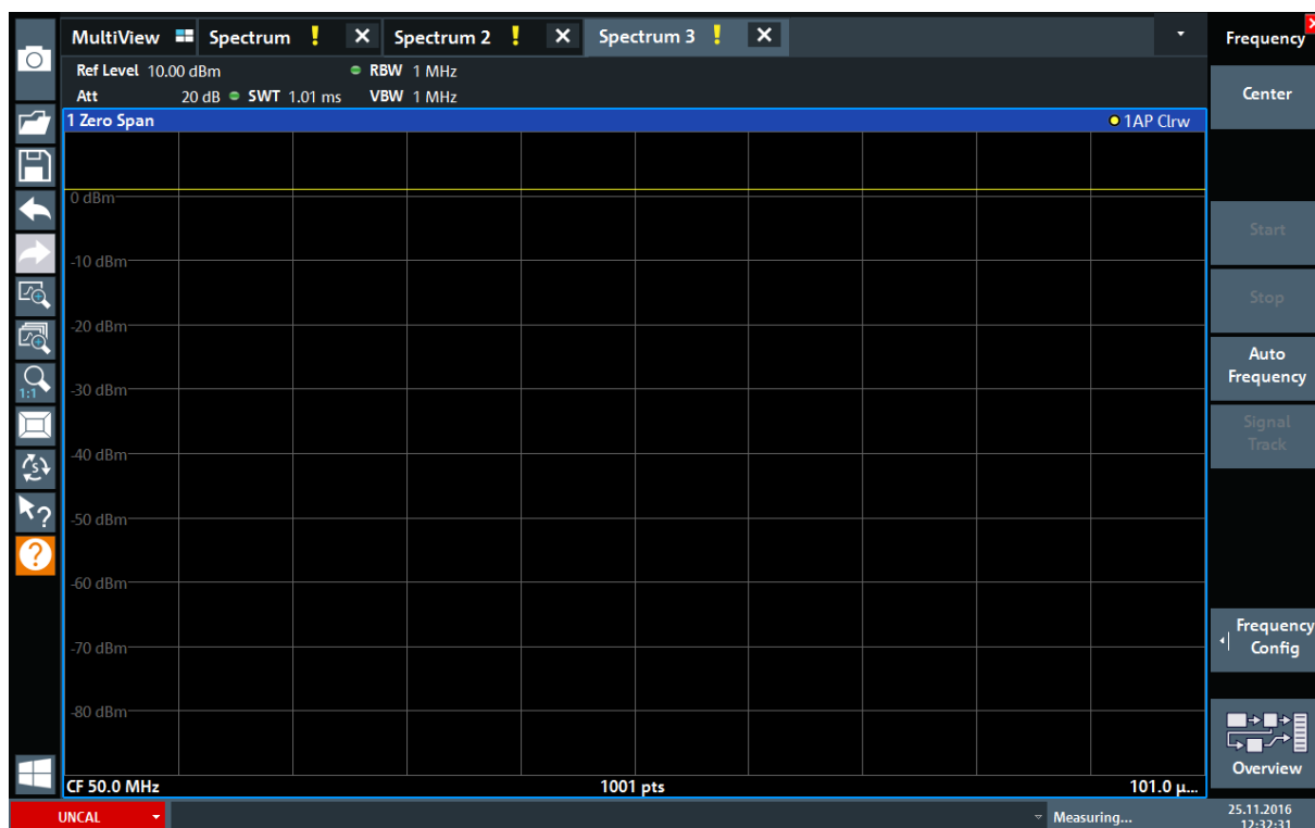
Figure 6-7: Time domain display of the calibration signal
