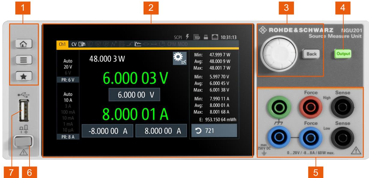
**Figure 6-1: Front panel of R&S NGU201 model**
