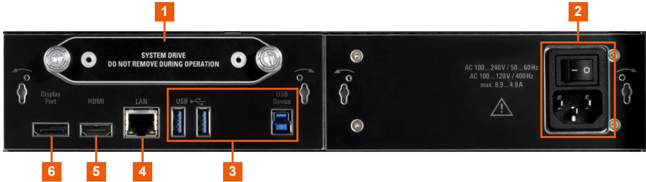
Figure 4-5: Processing board connectors and power supply
