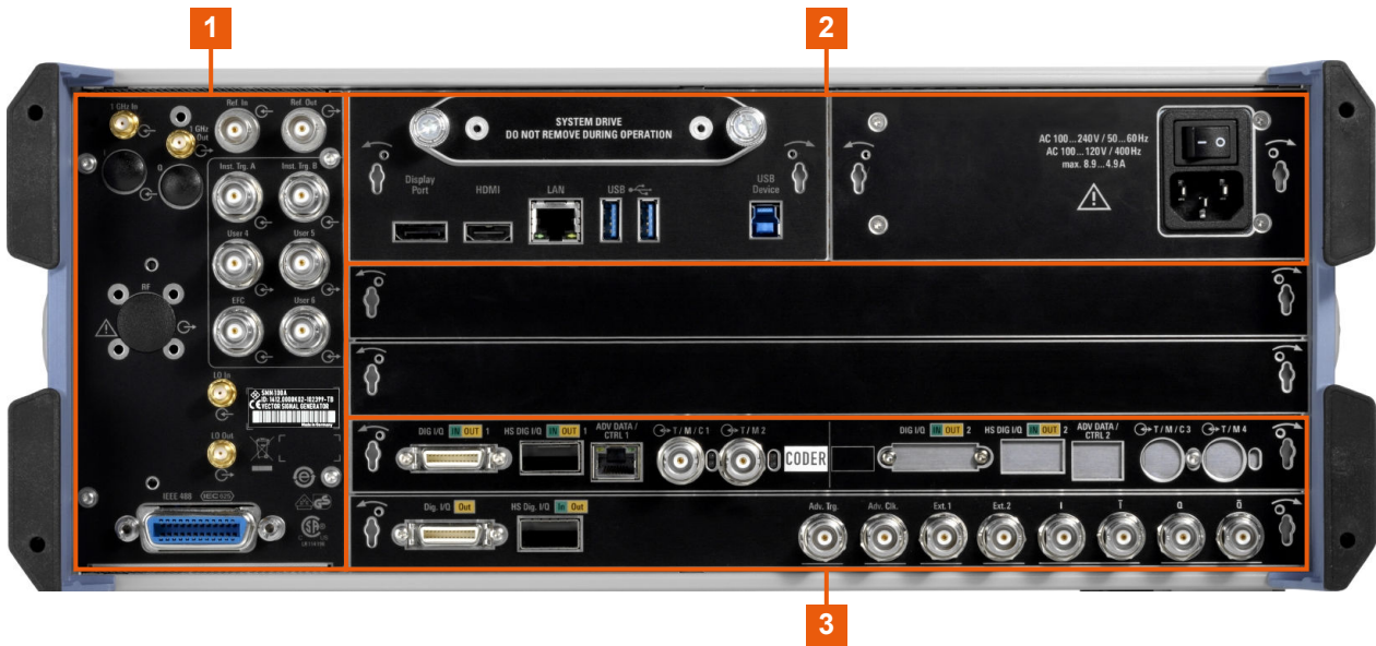
Figure 4-3: R&S SMM100A rear panel connectors
