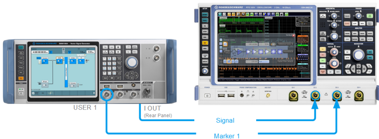
Figure 5-7: Simplified representation of a test setup for signal monitoring**
