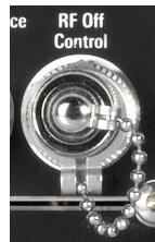
Figure 4-2: RF Off Control, terminated with attached Short
