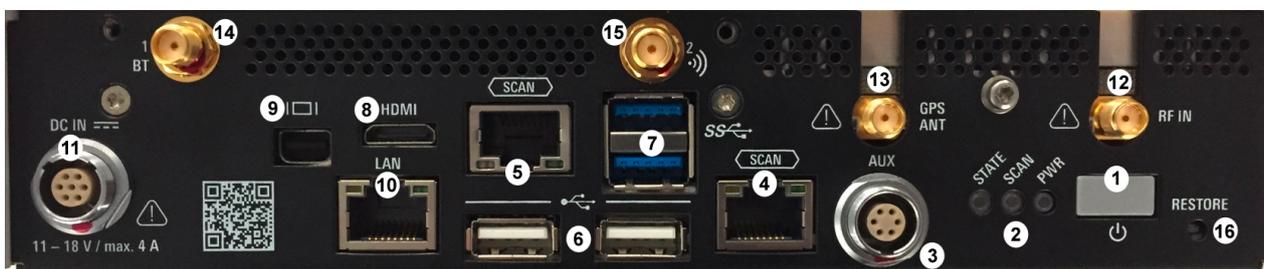
Figure 5-2: R&S TSMA - Rear Panel
