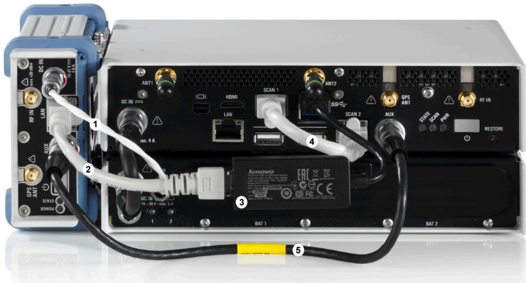
**Figure 4-20: Cabling of R&S TSME with R&S TSMA**
