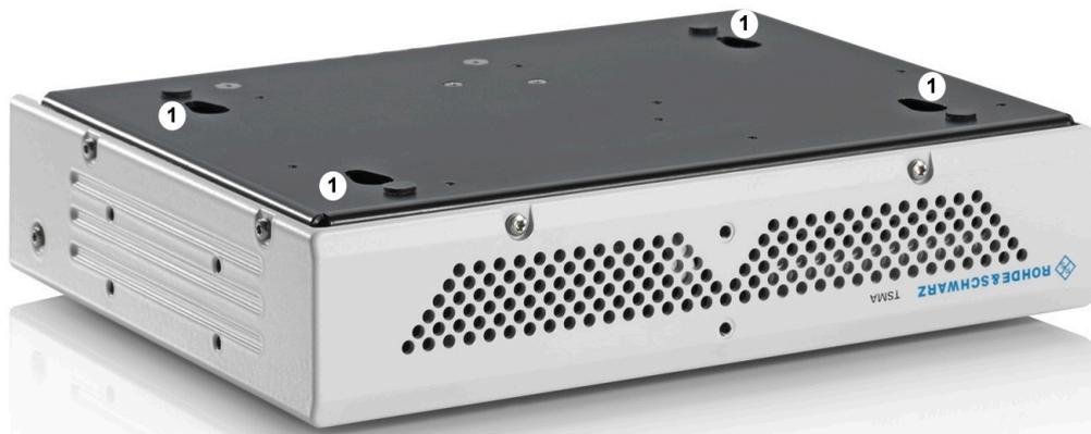
**Figure 4-8: R&S TSMA Base Unit (bottom side)**
