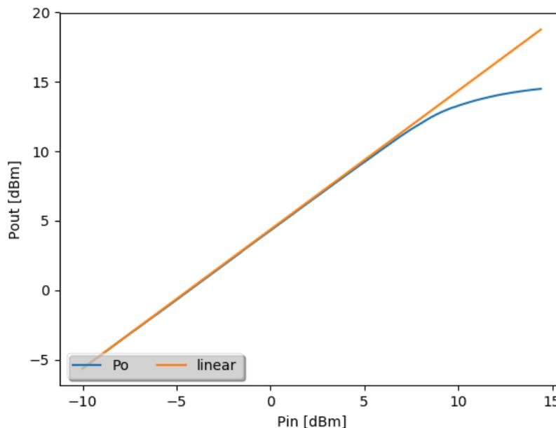
**Figure 2-1: Output power vs. input power of an amplifier**
