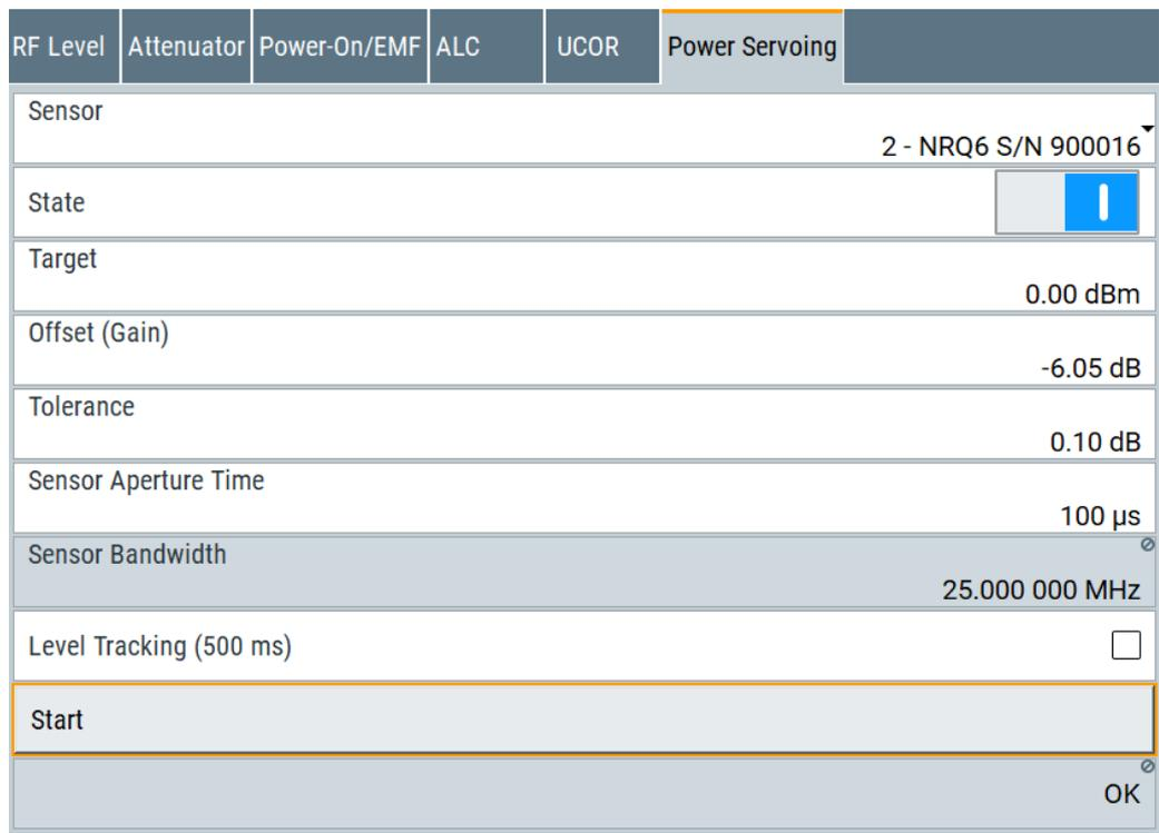
Figure 3-2: Power Servoing dialog of the SGMA GUI
