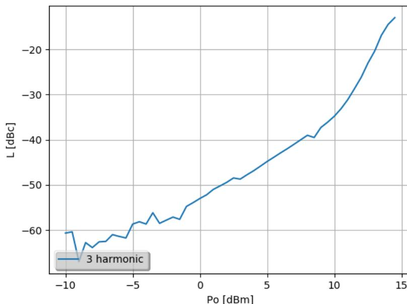
Figure 4-2: 3rd harmonic vs. output power measured with a spectrum analyzer
