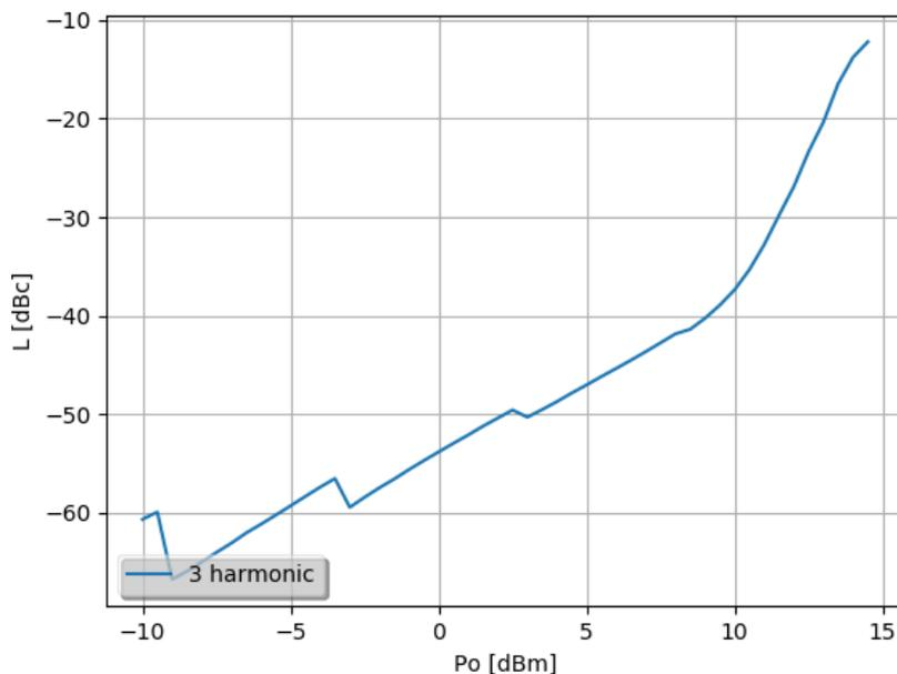
Figure 4-1: 3rd harmonic vs. output power measured with R&S NRQ6
