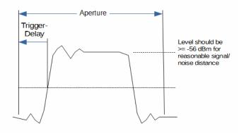
The selection of negative trigger delay and aperture time depends on the pulse form. Ideally, we can acquire at least 25 ns before the rising edge and up to 100 ns beyond the falling edge of the pulse.
