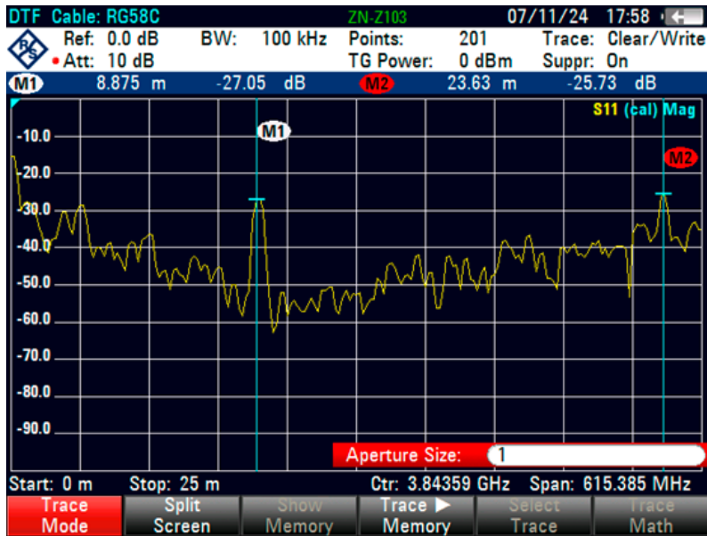
Figure 7-4: DTF measurement: The result shows that the cable had faults at 8.87 m and 23.6 m
