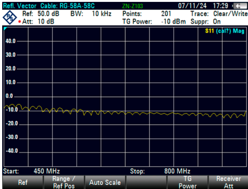
Figure 7-2: Return loss measurement on an RG-58C cable with source power at -10 dBm using an R&S®ZVH cable and antenna analyzer
