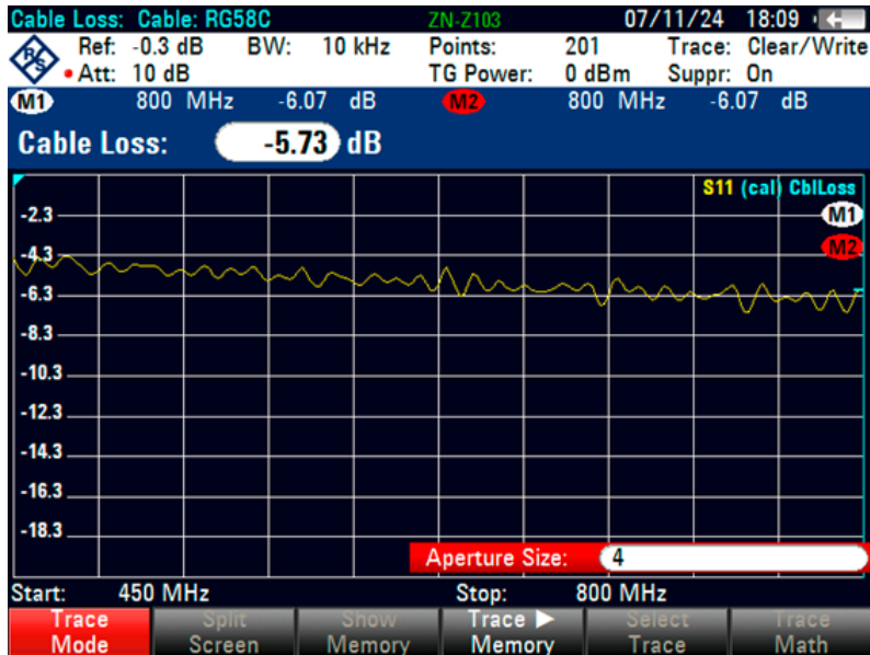
Figure 7-5: Cable loss measurement across a 25 m long cable
