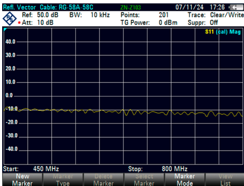
Figure 7-1: Return loss measurement on an RG-58C cable with source power at 0 dBm using an R&S®ZVH cable and antenna analyzer
