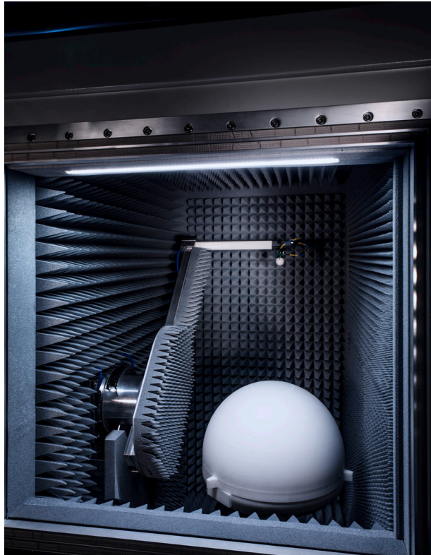
Figure 21: R&S®ATS1000 direct far-field test setup including temperature test solution
