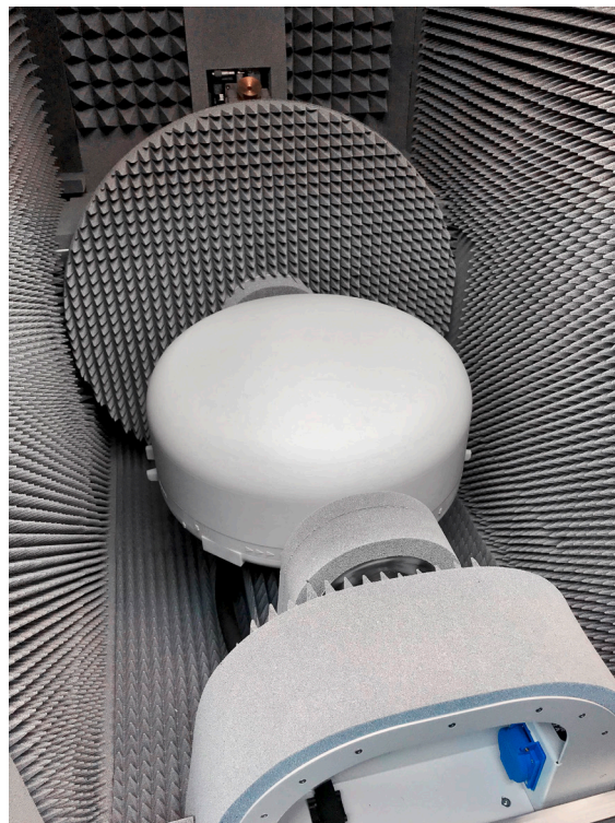
Figure 28: R&S®CATR-TEMP2 DUT enclosure for controlled environmental temperature conditions
