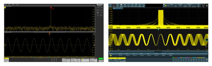
Fig. 15: Comparison of a modulated signal and an eye diagram on an oscilloscope with a slow update rate versus an oscilloscope with a fast update rate
