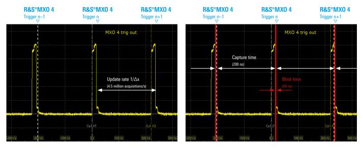
This example represents an ideal update rate measurement where the trigger out pulses are equally spaced. In reality, trigger out pulses will not always occur at regular intervals, as described later in this paper.
