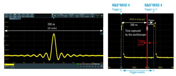
On the R&S®MXO 4 and R&S®MXO 5 Series oscilloscopes with a timebase setting of 20 ns/div, the instruments capture 200 ns each acquisition. We previously measured the minimum trigger rearm time to be 21 ns. For trigger events that are each spaced 250 ns apart with 200 ns per acquisition and a trigger rearm time of 21 ns, the R&S®MXO 4 captures 100% of trigger events. Increasing the test signal frequency shows a 100% trigger event capture rate up to 4.3 million acquisitions/s.
