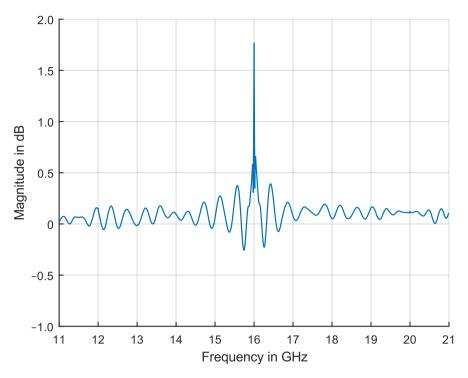
Measured frequency response, level = 0 dBm, RF output
