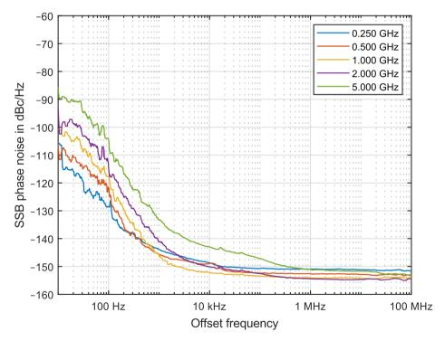
Measured SSB phase noise for a sine wave
