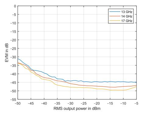
Measured EVM of a 2 GHz 5G NR signal, full allocation, SCS: 960 kHz, modulation: 256QAM, optimize EVM turned on, using the R&S®FSW signal and spectrum analyzer with the R&S®FSW-K575 I/Q noise cancellation option (IQNC with 50 iterations)
