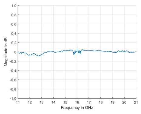
Measured level accuracy over frequency, level = 0 dBm, RF output
