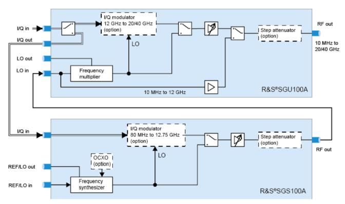
Functional diagram of R&S®SGU100A in combination with R&S®SGS100A signal generator.
