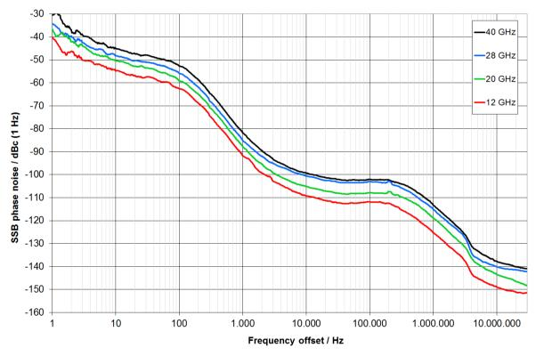
SSB phase noise in combination with R&S®SGS100A (meas.)
