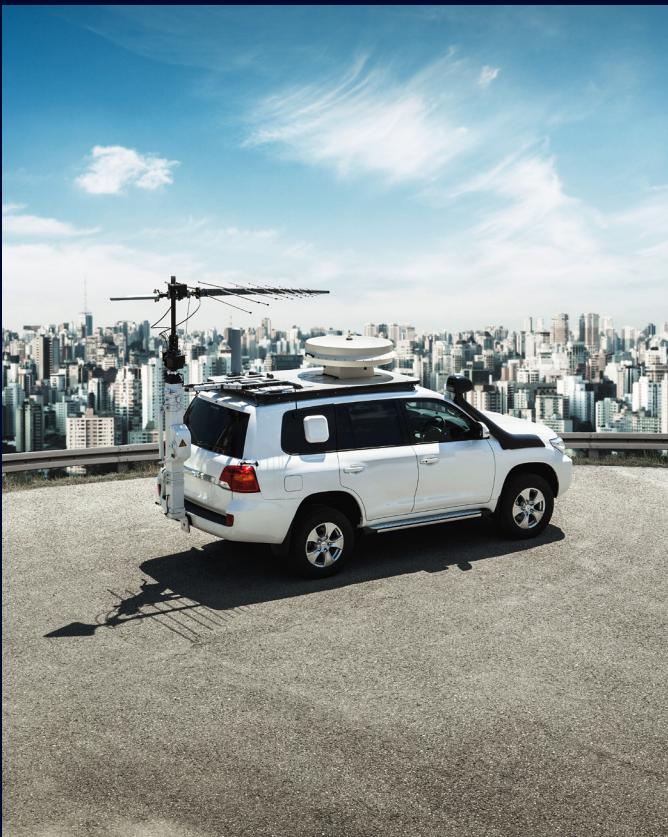
R&S®ESME installed in a mobile monitoring station
