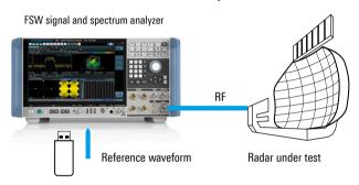
The R&S®FSW-K60P transient phase noise extension adds phase noise measurements to individual chirps or hops in the measurement results.
