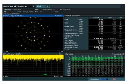
DVB-S2X signals use different modulation schemes for the payload and the header sections of the frame. The different types of modulation can be analyzed using the R&S®FSW-K70M and R&S®FSW-K70 options. The screenshot above shows a DVB-S2X signal using 64APSK for the payload and QPSK for the pilot channels.
