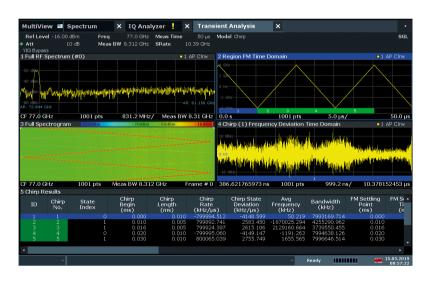
Analysis of an FMCW signal with the R&S®FSW-K60C option and 8.3 GHz analysis bandwidth
