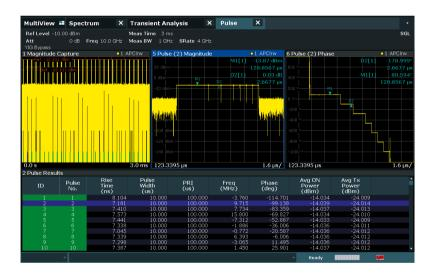
Equipped with the R&S®FSW-K6 pulse measurements option, the FSW delivers pulse parameters at the touch of a button.
