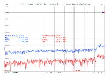
The sensitivity of the R&S<sup>®</sup>ZNA26/R&S<sup>®</sup>ZNA43 receivers can reach –150 dBm (lower frequency end, typical, at 1 Hz IFBW, direct channel access/reversed coupler, receiver step attenuator in 0 dB position). The sensitivity of the b1 and b2 receivers is increased further by using the R&S<sup>®</sup>ZNAxx-B302 and R&S<sup>®</sup>ZNAxx-B501 preamplifiers.
