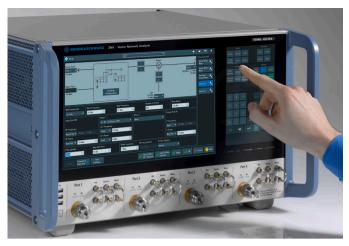
Control of the R&S<sup>®</sup>ZNA via touch panel. Users benefit from all-in-one dialogs, which provide a clear overview of all key parameters and help to keep track of the overall measurement configuration.
