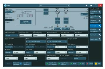
All-in-one dialog for intermodulation measurement on a double converting receiver
