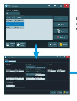
Based on the DUT type, the user is prompted to select and configure the desired measurements in a step-by-step process. The required channels and traces, e.g. for measuring LO feedthrough, are automatically created.
