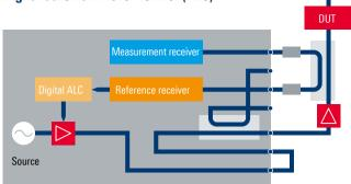
ALC operation: in a high-power setup with an external preamplifier and a directional coupler, the source power is controlled to match the preamplifier output power. This compensates for drift effects, making the output power very precise and stable.
