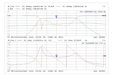
calculates the group delay and the relative phase. The frequency drift and frequency modulation of the DUT's internal LO do not affect the measurement accuracy as long as the frequency deviation lies within the analyzer's IF bandwidth used for the measurement.
