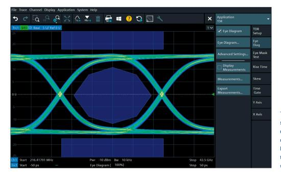
The R&S<sup>®</sup>ZNA-K20 option offers versatile signal integrity measurements, e.g. eye diagrams with a mask to verify compliance with relevant requirements. It can also be used to determine the transmission characteristics of signals with jitter or noise.
