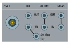
R&S<sup>®</sup>ZNAxx-B16 front panel jumper position required for direct source monitor access (R&S<sup>®</sup>ZNAxx-B161/-B163)
