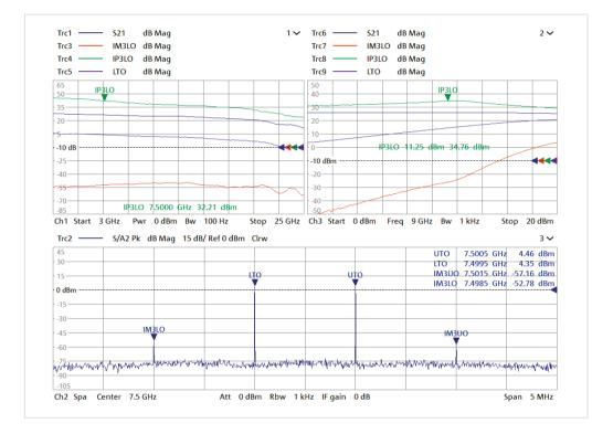
Comprehensive amplifier characterization, including intermodulation products (IP), IP versus frequency, spectral measurements and other quantities
