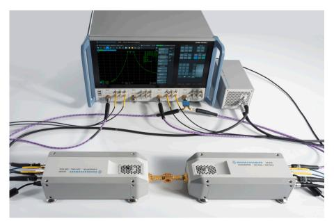
Setup for mmWave measurements with an R&S<sup>®</sup>ZNA43 and two R&S<sup>®</sup>ZC330 mmWave converters WM-864
