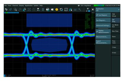
Eye diagram mask test with synthetic signal predistortion
