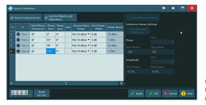
GUI for entering dedicated port specific values for phase and power. In automatic true differential measurement mode, users can enter parameters for phase and magnitude imbalance sweeps.
