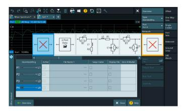
The R&S<sup>®</sup>ZNA comes with a choice of predefined matching networks whose values can be edited. If values are changed, the R&S<sup>®</sup>ZNA will immediately recalculate the network and embed the DUT in the new network in real time.
