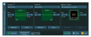
For in-fixture and PCB tests Rohde & Schwarz offers advanced coupon based deembedding options, supported by a smart configuration wizard.
