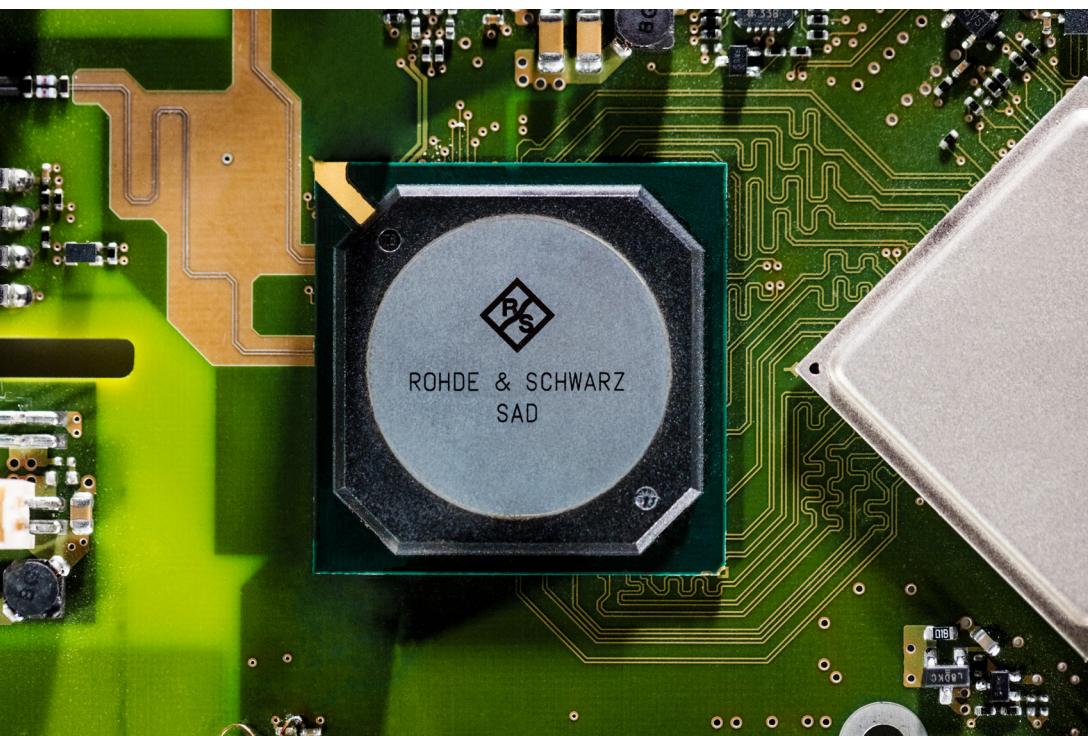
The Rohde & Schwarz designed 10-bit A/D converter ensures highest signal fidelity at highest resolution
