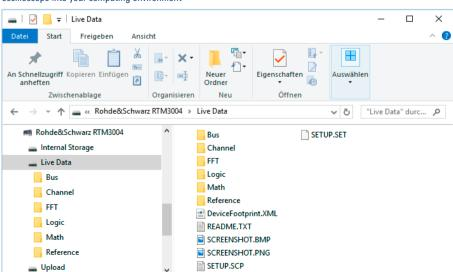
With the USB MTP implementation, you can easily access live channel data and screenshots and integrate the oscilloscope into your computing environment
