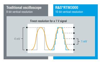
One example is the characterization of switched-mode power supplies. The voltages across the switching device must be determined during the on/off times within the same acquisition. For precise measurements of small voltage components, a high resolution of more than 8 bit is essential.
