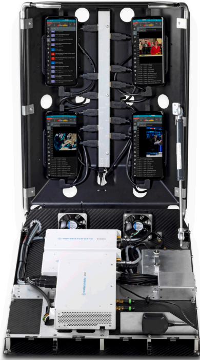
Freerider CORE with mounted mobile phones and scanner.
