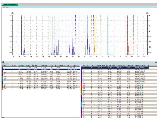
CIR View shows the channel impulse response (CIR) and all parts of the multipath propagation (echoes) together with a cell's cyclic prefix.
