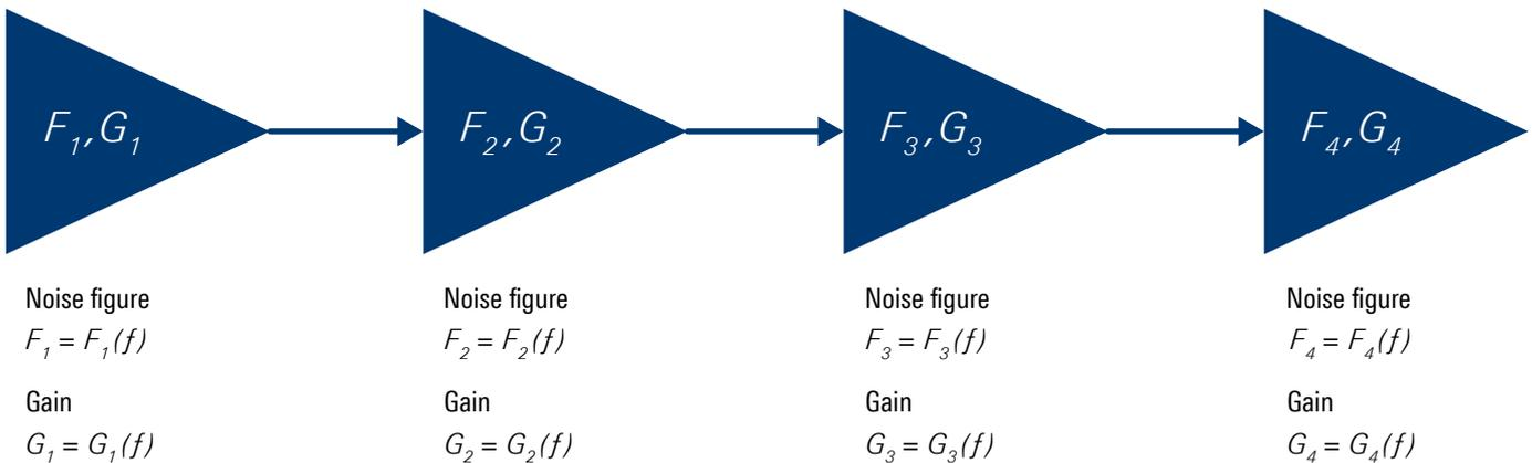
$$F_{total} = F_1 + \frac{F_2 - 1}{G_1} + \frac{F_3 - 1}{G_1 G_2} + \frac{F_4 - 1}{G_1 G_2 G_3} + \dots$$
