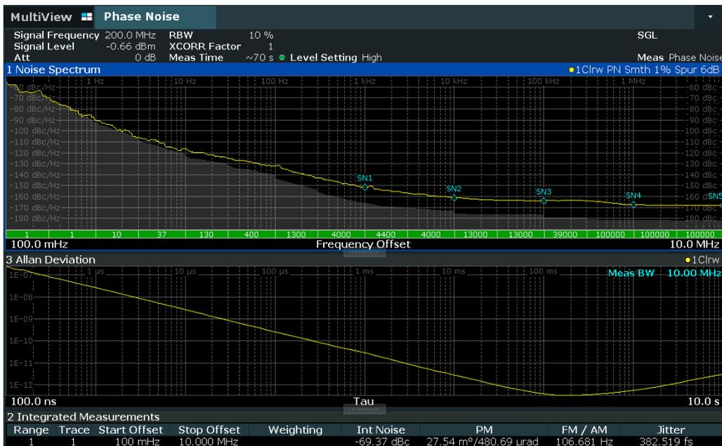
The R&S®FSPN calculates the Allan variance based on the phase noise measurement (upper window). For example, an offset range of 100 mHz to 10 MHz corresponds to a time-domain display of 100 ns to 10 s.
