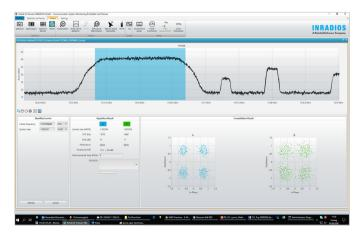
Detection and classification of symmetric carrier-in-carrier signals
