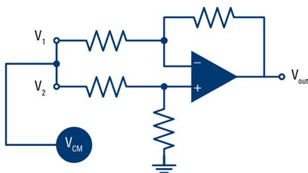
$$V_{out} = A_{dm}(V_1 - V_2) + A_{cm}(V_{cm})$$
