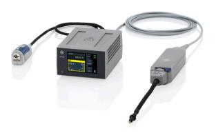
The R&S®RT-ZISO isolated probing system lets you connect to any oscilloscope with a BNC or SMA interface. The probe receiver comes with a touchscreen display to control and view probe system settings, for easier control of the probe range and offset settings while also indicating the connected probe tip.
