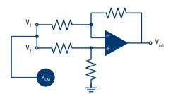
$$\begin{aligned} &V_{out} = A_{dm}(V_1 - V_2) + A_{cm}(V_{cm}) \\ &CMRR = \left(\frac{A_{dm}}{|A_{cm}|}\right) \\ &CMRR_{dB} = 20log_{10}\left(\frac{A_{dm}}{|A_{cm}|}\right) \end{aligned}$$
