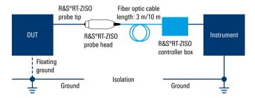
The signal transmission from the probe head to the probe receiver box is made with an optical connection and the necessary power supply for the probe head is transmitted over fiber. The probe head does not need an external power source, limiting the possibility of another common mode loop, unless an isolated source such as a battery is used.
