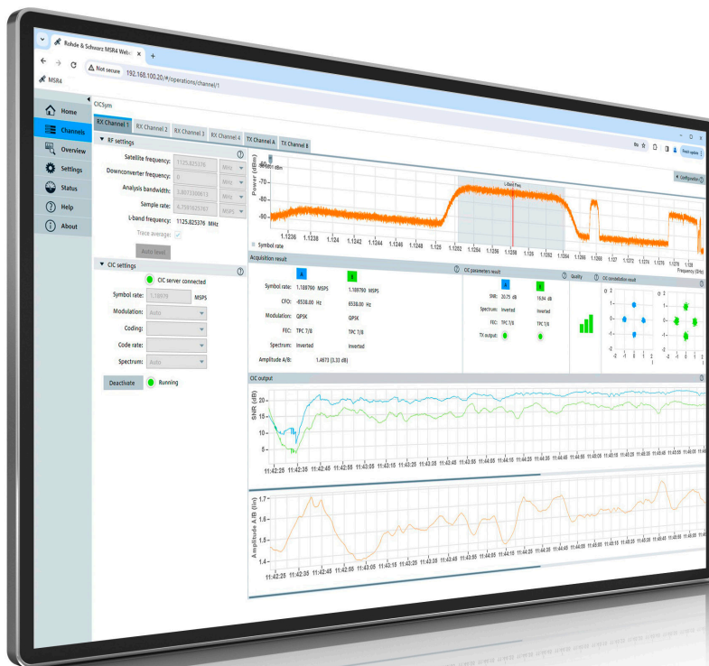
The R&S®MSR4-142x carrier-in-carrier symmetric splitting options are seamlessly integrated in the R&S®MSR4 GUI.
