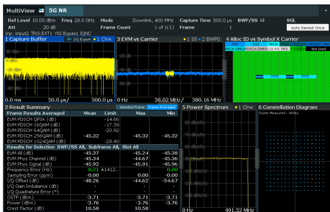
Measured EVM for a 400 MHz 5G NR signal, 28 GHz carrier frequency
