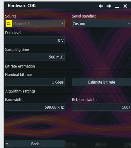
The configurable CDR of the R&S®RTO6 supports data rates up to 6 Gbps for data eye analysis.
