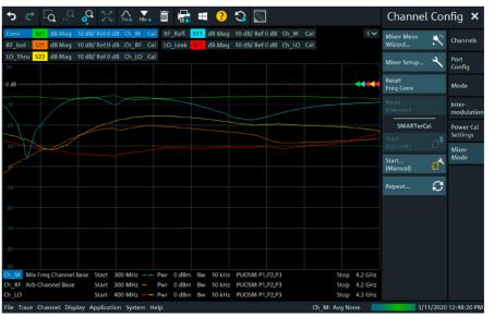
intermodulation measurements. This feature boosts measurement speed by a factor of up to 10 compared to setups using an external generator. Plus, it significantly simplifies the test setup.
