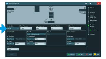
Based on the selected type of DUT, the wizard guides the user step by step to the desired measurement setup.
