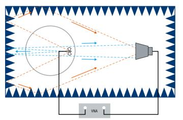
The time domain site VSWR (TD S<sub>VSWR</sub>) measurement in line with ANSI C63.25 is a fast and precise method for validating fully anechoic rooms (FAR). It involves a series of impulse response measurements, which are performed by a 2-port R&S<sup>®</sup>ZNB20 or R&S<sup>®</sup>ZNB26 equipped with the R&S®ZNB-K2 option, plus an R&S®HF907 double-ridged waveguide horn antenna. The R&S<sup>®</sup>ZNrun software can be used to automate the test sequence.
