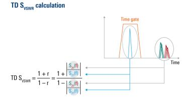
TD S<sub>vewp</sub> measurements with a vector network analyzer
