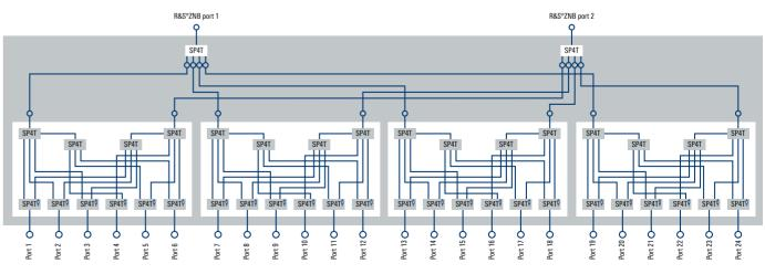
loss, maximum accuracy and a large number of ports. The R&S°ZN-Z84, R&S°ZN-Z85 and R&S°ZN-Z86 cover frequencies up to 8.5 GHz, 20 GHz and 26.5 GHz respectively. The base units each come with six outputs. The R&S°ZN-Z84 and R&S°ZN-Z86 switch matrices can be expanded to offer up to 24 outputs by adding further ports in groups of six. The R&S°ZN-Z85 is available with two inputs and six outputs or with four inputs and 12 outputs.
