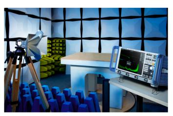
R&S®ZNB20 equipped with the R&S®ZNB-K2 time domain analysis option, together with an R&S®HF907 double-ridged waveguide horn antenna, provides an ideal solution for fast and accurate site validation measurements using the TD S..... method in line with ANSI C63.25.
