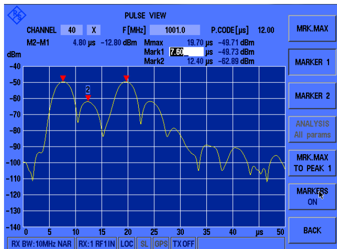
Time domain analysis of direct and reflected pulses.
