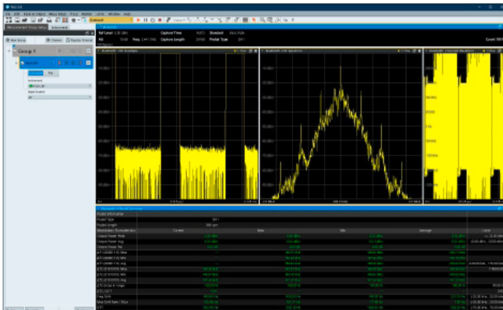
Analysis of a Bluetooth® (BR) signal with a detailed result summary display.
