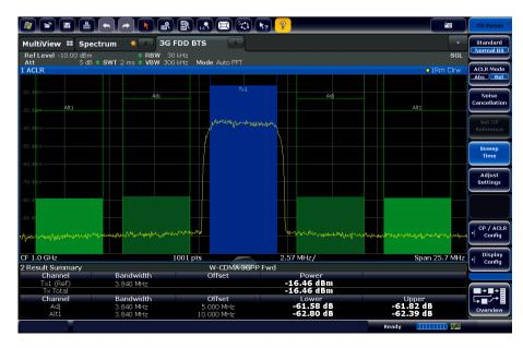
Adjacent channel leakage ratio (ACLR) measurement of a 3GPP WCDMA signal
