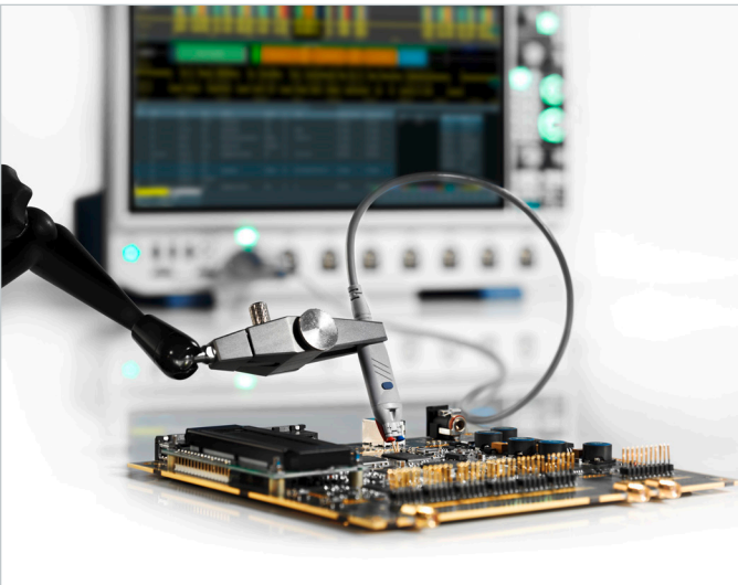
R&S®RT-ZAP 3D probe positioner in use with the R&S®RT-ZD30
