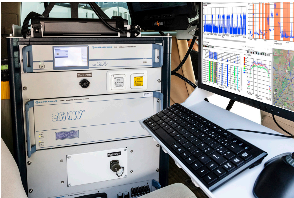
Fig. 2: The R&S®ESMW mounted in a 19-inch rack in a measurement vehicle.
