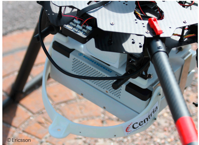
Drone based testing with an R&S®TSM 6B.
