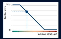
Fig. 3: Conversion of technical measured values into dimensionless points with saturation areas provides a simple simulation of human perception.
