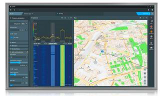
R&S®CEPTOR provides a real-time overview of the electromagnetic environment and can log any emission between 8 kHz and 20 GHz.
