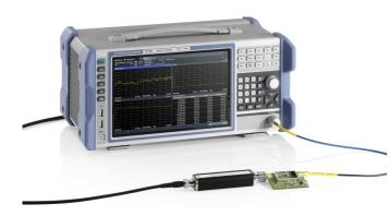
Measure noise figure and gain of amplifiers with an R&S°FPL1000 with the R&S°FPL1-K30 option and a noise source.
