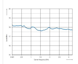
The high output power of typ. > +17 dBm enables measurements on DUTs such as mixers that require a highlevel for the local oscillator.
