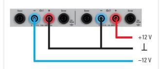
The circuitry of each single channel is completely isolated from the others; there is no connection to chassis ground. This makes it easy to combine the channels to drive balanced circuitries that might need +12 V/-12 V, for example, and avoids ground problems in complex DUTs.
