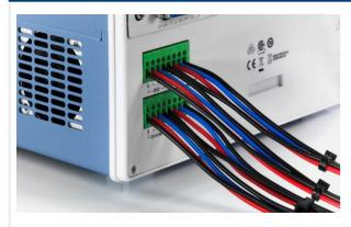
$\label{eq:connections} \mbox{ for all channels} - \mbox{ including sense} - \mbox{ are also provided on the rear panel}$
