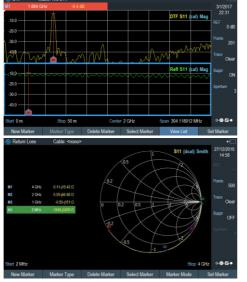
Standard measurements include distance to fault, return loss, one-port cable loss, reflection ( $S_{11}$ ). Result formats of  $S_{11}$  reflection measurements : magnitude, SWR, Smith chart, phase, etc.
