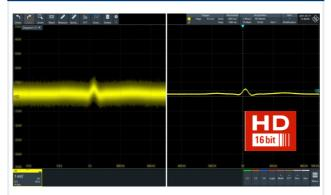
The unique digital trigger system from Rohde & Schwarz uses the sampling points of the A/D converter in the acquisition path so the trigger system's input data is identical to the displayed signal. The trigger system runs in high definition (HD) mode with up to 16-bit vertical resolution. This results in very high trigger sensitivity. You can reliably isolate even the smallest signal details.
