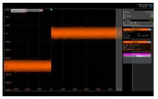
The LeCroy HVD3220 probe has up to 12 times more noise than the R&S\*RT-ZHD. High noise reduces the accuracy of measurements and makes it difficult to see small details and trigger on them.
