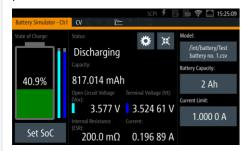
The charging behavior of a battery can also be simulated, for example when designing battery chargers. In this application, the R&S®NGM200 is used in sink mode.
